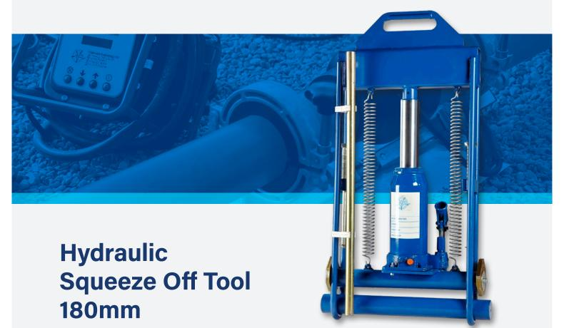
Designed for flow control or temporary closure of large size pipes. Generating a force of 15 tonnes the hydraulic jack will close PE pipe of any standard wall thickness within the size range.
