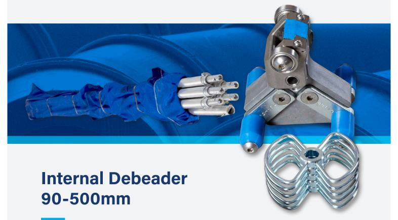
The Internal Debeader easily removes the bead formed by the butt fusion process of pipe welding during the cooling cycle. The rod sections can be joined together to reach weld beads of up to 24m.
