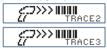
The option to scan up to three traceability barcodes is permitted. If no traceability barcode is to be scanned press the green button to continue. After each traceability barcode is scanned the option to exit this stage is available by pressing the green button, otherwise scan the next traceability barcode.
