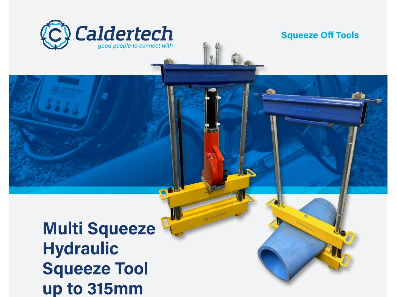
Designed for flow control or temporary closure of large size pipes. Generating a force of 25 tonnes the hydraulic jack will close PE pipe of all sizes up to 315mm SDR11.
